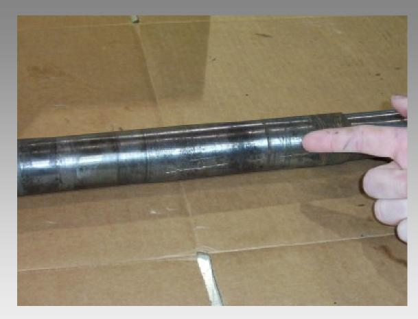
APO Will Metalize & Machine Sleeve to Original Factory Tolerance
